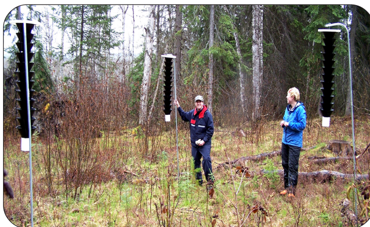
Lindgren funnel traps placed in a 3 trap cluster
